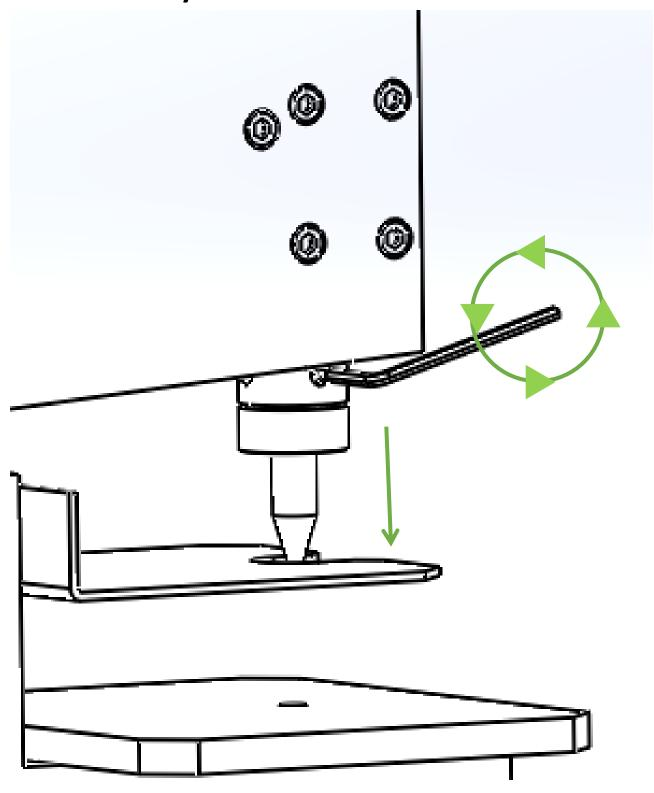
Step 1: Use a 2.5mm L-Wrench, loosen the bolt assembled at the bottom of Ram Piston about 1 turn counterclockwise.
