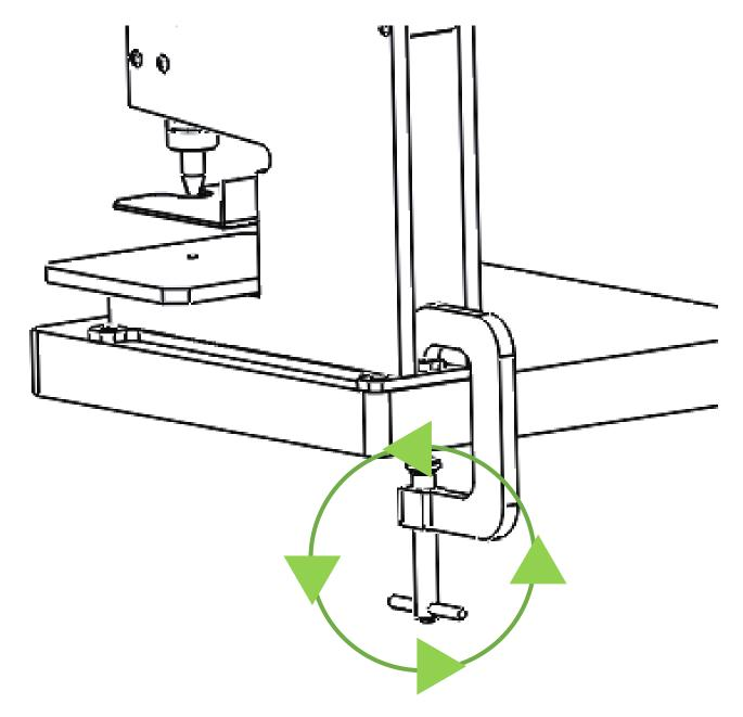
Use the included C-Clamp to attach the back of the HDT02-K to the workbench
