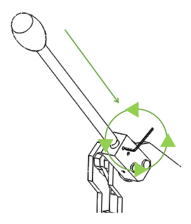
Step 1: Use a 2.5mm L-Wrench, loosen the 2 bolts assembled in the lever fixing block about two turns counterclockwise
